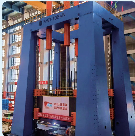
10,000-ton multi-functional testing system
